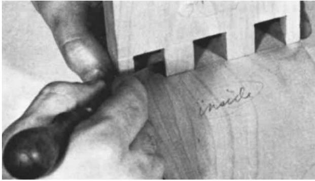
scriber tight against the sides of the pins. From the outside the tool tends to follow the grain away from the side of the pin.
