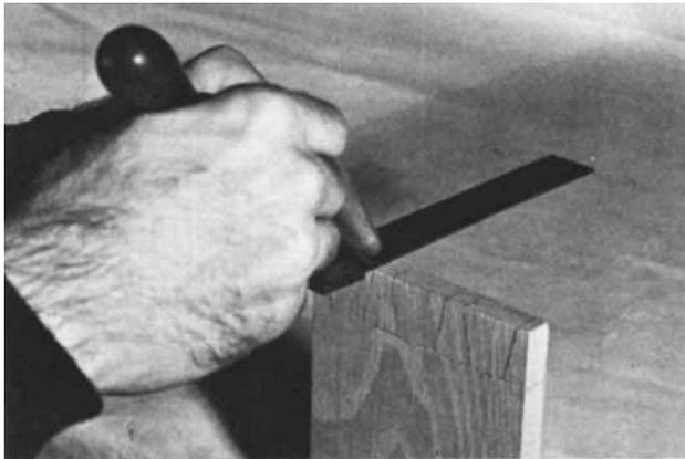
same way as when laying out pins for through dovetails except you will be working on the outside of the drawer side rather than on the end grain of the drawer front.
