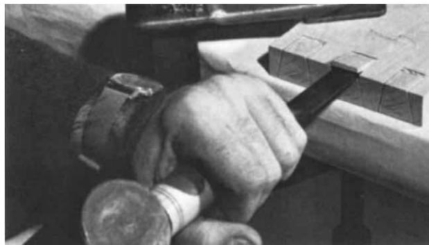
When you are making the vertical cuts across the grain at the marking gauge line, it helps to tip the chisel forward a few degrees. This is called undercutting and if done when chiseling from both sides it will result in a shallow, concave surface in the end grain between the pins. Remember that
