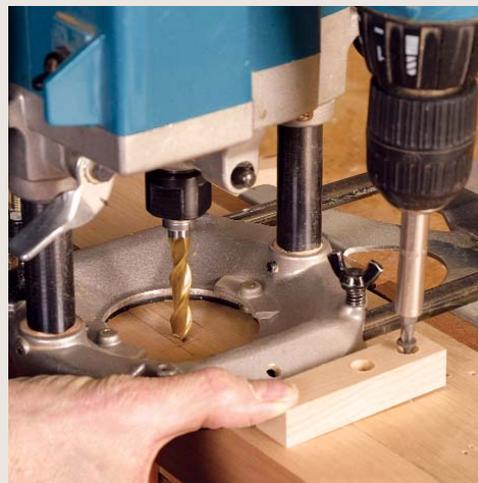
**Stop blocks establish the mortise length.** Stop blocks on each side of the router base limit the travel of the base.
