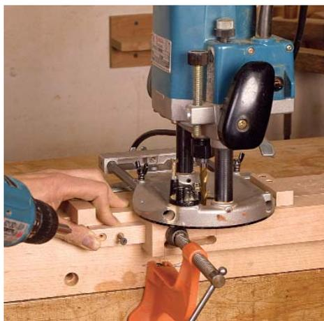
The diameter of the router bit determines the width of the mortise. For example, a  $\frac{1}{4}$ -in.-wide mortise is cut with a  $\frac{1}{4}$ -in.-dia. bit; and a  $\frac{3}{4}$ -in.-wide mortise is cut with a  $\frac{3}{4}$ -in.-dia. bit. You also could choose a mortise width that requires moving the router over and taking extra passes to widen the opening. But because straight bits are available in so many sizes, you can usually find one to match the mortise width you need.
