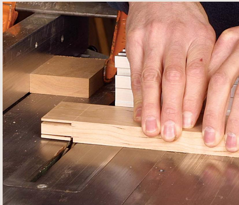
**Use the miter gauge and a stop block.** For consistent tenon shoulders, clamp the stop block to the rip fence and make the shoulder cuts using a miter gauge.
