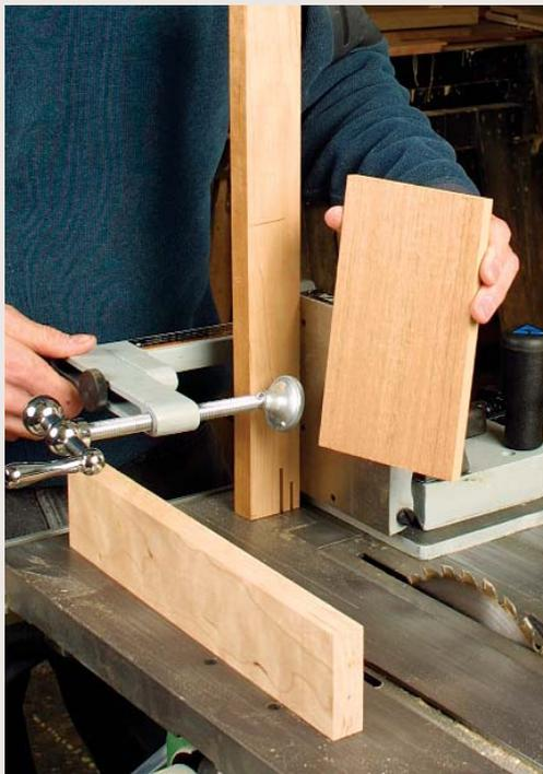
**Spacer makes tenons of uniform thickness.** The spacer should be a hair thinner than the width of the mortise plus the width of the sawkerf.
