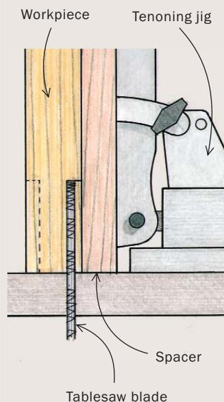
**Clamp the spacer in the jig and against the scrap stock in back.** Adjust the jig to line up with the tenon mark, then cut the first cheek.
