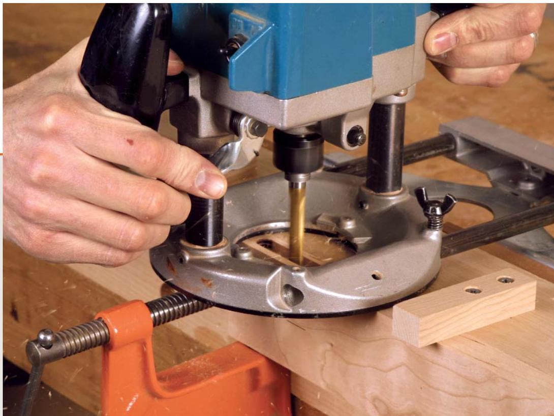
**Take light cuts until you reach the final depth.** To produce smooth, straight-sided mortises, make multiple passes with the router, with each pass removing no more than  $\frac{1}{32}$  in. of stock.
