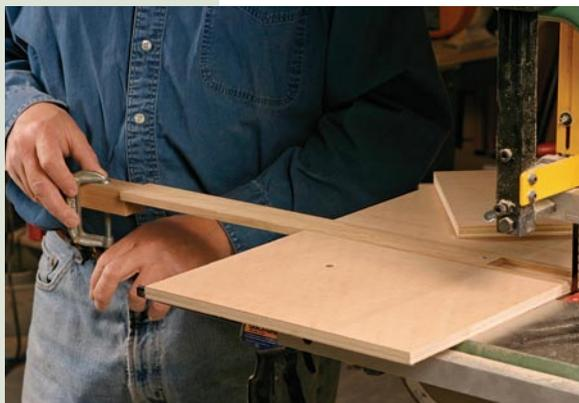
**Attach the stop.** After measuring the distance from the pivot point to the blade (circle radius), clamp the stop on the underside of the arm at the end of the guide track (above left).
