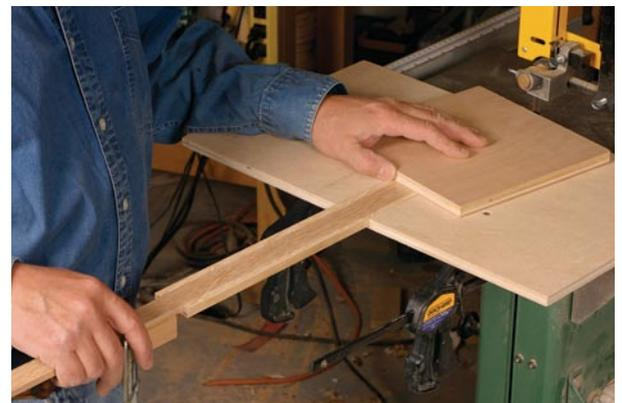
**Spiral into the circle.** With the saw running, gently push the arm forward while rotating the stock into the blade (above right). Once the stop reaches the end of the guide track, the blade starts to cut the actual circle (right).
