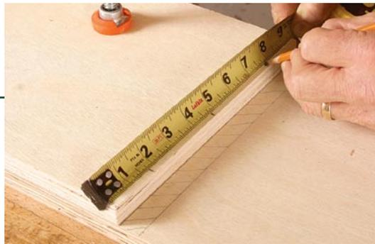
**Layout trick.** To start, mark out the shelf location on the case side and clamp the actual shelf along one of those lines. You are now set up to cut both sides of the biscuit joint.
