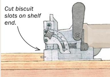
**Just butt and cut.** With the joiner base on the side piece, cut the biscuit slots in the end of the shelf (above). Reposition the joiner so the base butts against the end of the shelf, and cut the mating slots in the side piece (below).
