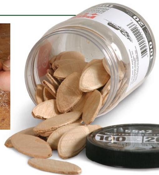
**Simple and efficient.** An adjustable stop on the joiner (left) controls the depth of cut to match each of the common biscuit sizes—0, 10, and 20. A biscuit swells in thickness (right) when wet glue hits it, helping to anchor the joint. So store biscuits in a sealed jar to keep out moisture.
