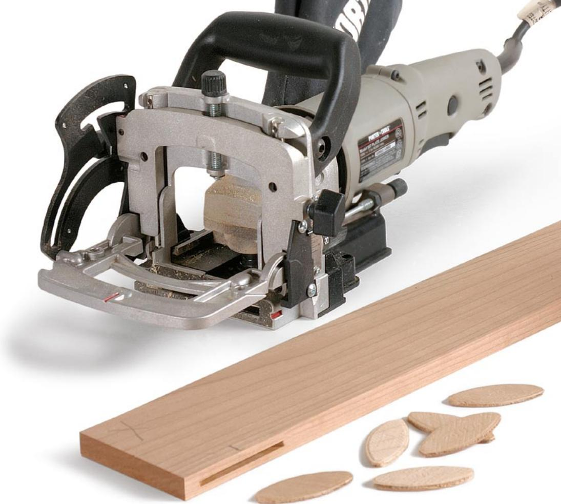
called a biscuit joiner or a plate joiner. To make a joint, use the tool to cut a shallow slot in each of the mating parts. Then, after adding glue to each slot, insert a thin, football-shaped biscuit into one slot. A little more than half the biscuit's width goes into the slot; the other half sticks out. To complete the joint, just slip the mating slot onto the "tenon" and clamp the parts together.
