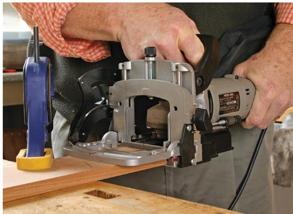
**Center the cutter on the stock's thickness.** With the fence flat on the workpiece, adjust its height to locate the cut. To make the cut, simply align the joiner with the single layout mark, start the tool, and push the joiner's body forward.
