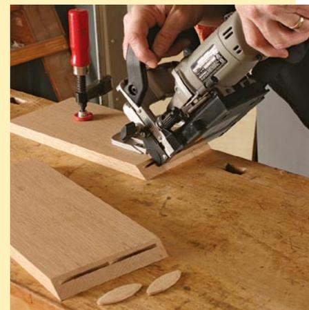
Setting the fence to 45° allows the joiner to cut a slot in the end of a mitered workpiece. Align the joiner for a cut toward the inside of the miter, so there is plenty of material in which to sink the slot.
