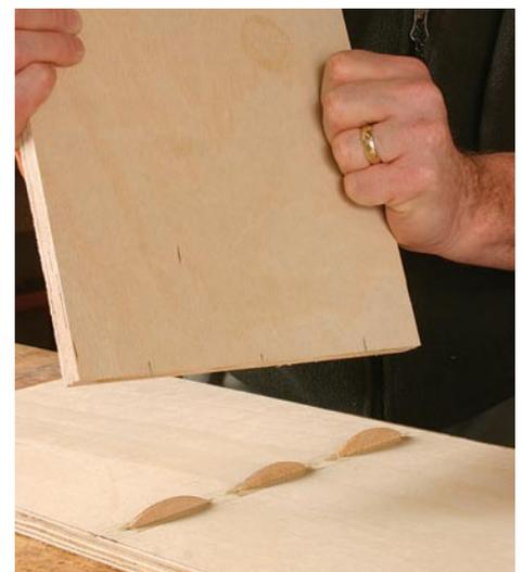
**Join the parts.** Apply glue to the slots and biscuits, then fit the shelf to the side pieces and add clamps.
