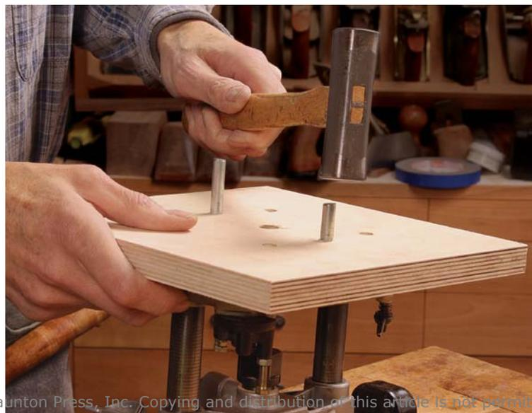
**Pins center the router.** Add some glue, drive in two 3/8-in. dowels or metal pins, and the jig is done.
