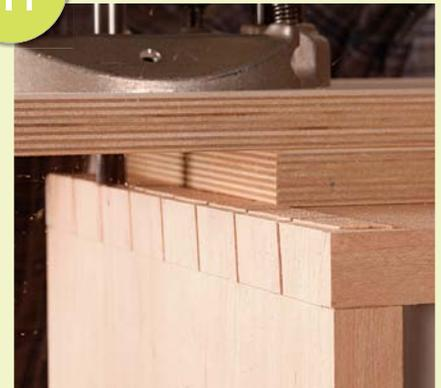
A bottom layer with a straight front edge is great for flush-trimming dovetails.
