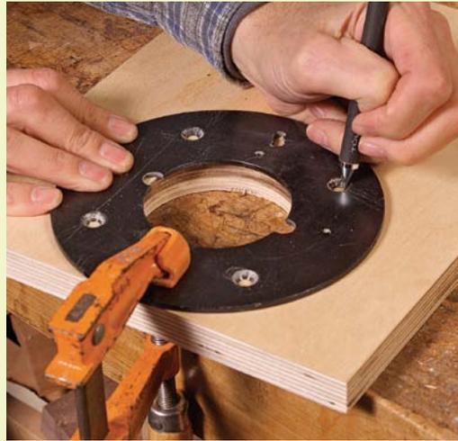
**For better balance, a bigger footprint.** An oversize base gives you greater control when routing an edge with large profile bits. Use the router's plastic sub-base as a template for drilling the mounting holes.
