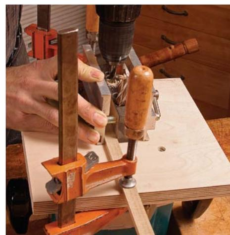
**Rotate the jig.** After drilling the first hole, spin the jig 180° to locate the opposite hole.
