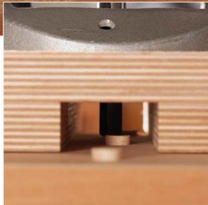
**Sure-footed.** The base straddles a series of screw-hole plugs, for example, with the twin support rails preventing the bit from tipping into the work surface.
