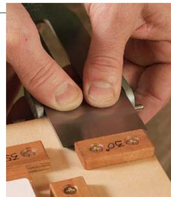
**Best value.** For less-expensive guides, make a setup board so that you can quickly set the protrusion of the blade for common angles. To do so, set up the guide for a given angle (left), then position a stop block (center) so you can return the guide quickly and positively to the same exact angle in the future (right).
