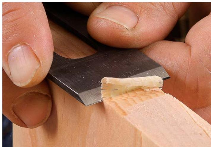
**The proof is in the pine.** A sharp chisel or plane blade will slice end-grain pine without tearing the fibers, leaving a glass-smooth surface.
