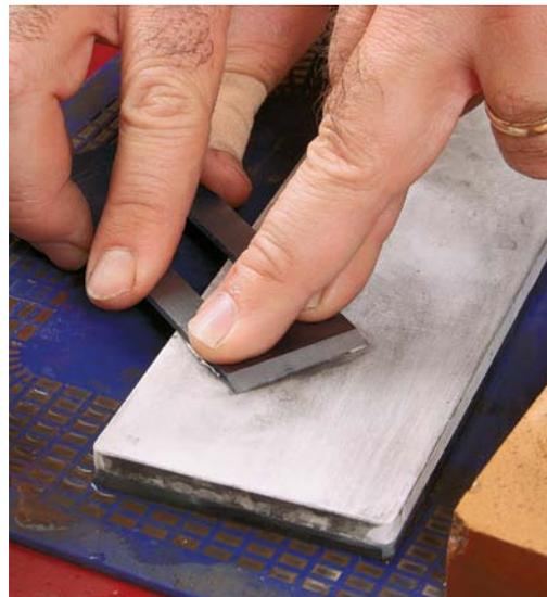
**Back to the back.** Take the blade out of the guide and take a few quick strokes on your finest stone to remove the burr that formed there as you honed the bevel.
