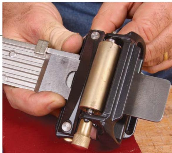
**Best overall.** The Veritas Mk. II honing guide comes with an attachment that locks in a wide variety of bevel angles (above left). A stop sets the angle (right) and a lip along one edge ensures that the blade is square to the jig. Also, the wide roller is very stable.
