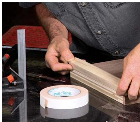
**Attach straightedges flush.** With the case sides cut to their final dimensions, attach straightedges flush to the edges of the workpieces (above) with double-sided tape (use thicker carpet tape). The other sides of the straightedges are cut at 45° so they can serve as clamping cauls during assembly.
