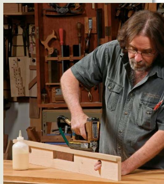
**Pop, pop.** Attach the two pieces with a bead of glue and a few nails (or countersunk screws).
