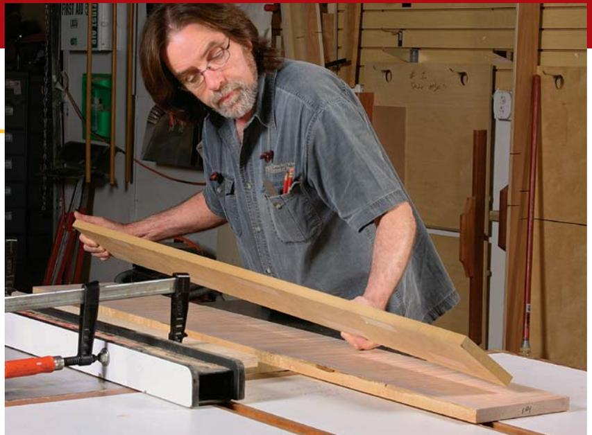
**Set up for a flush cut.** Use a ruler to align the edge of the L-fence with the outer edge of the teeth. The L-fence should be a little above the blade, and parallel to the table.
