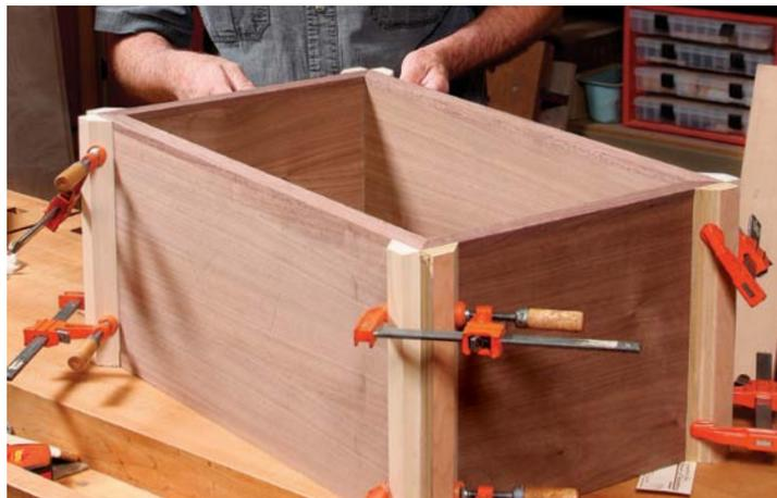
**Perfect miters come together quickly.** The clamping cauls make glue-up a breeze. When the glue sets, remove the cauls. A solvent rag cleans up any lingering residue from the double-sided tape.
