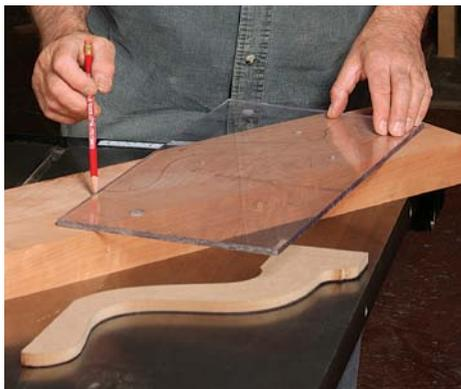
**Two templates.** Trace the leg pattern onto a square Lexan template. Then use the clear template to locate a leg on the blank and mark the straight edges.
