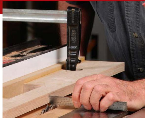
**Adjust the rip fence.** The width of the exposed dado set establishes the width of the rabbet. Measure from the edge of the L-fence to the outside of the blade's teeth.
