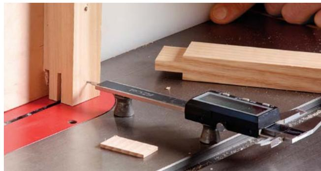
**Add magnets and make machines digital.** Use these standoff magnets from Lee Valley ([leevalley.com](http://leevalley.com)) to attach calipers to a metal surface, and then use the depth rod to make precise adjustments to fences, jigs, and more.
