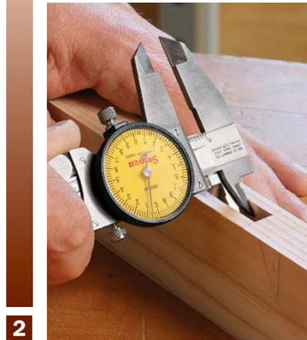
**Inside for width.** Use the inside jaws to find out exactly how wide a mortise is before cutting the tenon. They are also great for positioning a jig on a workpiece, and dozens of other tasks.
