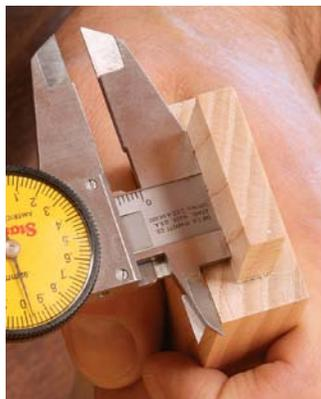
**Measure or mark.** The step lets you use the end of the jaws as a depth stop of sorts, for measuring distances (left). You can also slide the tool along an edge for marking and scribing (right).
