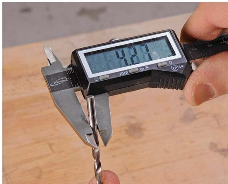
**Dial in the bits.** Fractional drill sizes can be confusing. Keep it simple by using the decimal scale to pick the right bit.
