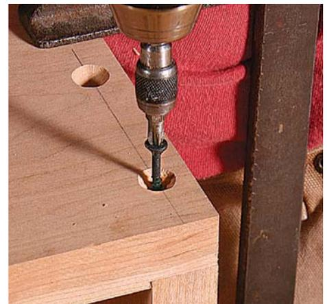
**Then drive the screw.** Accurate, tight, split-free screw joints result from proper predrilling.
