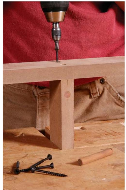
Screws don't grip well when you are screwing into the end grain of a piece of wood, or into the edge of a piece of MDF or plywood. To solve the problem, insert a dowel in the lower board and drive the screws through it.
