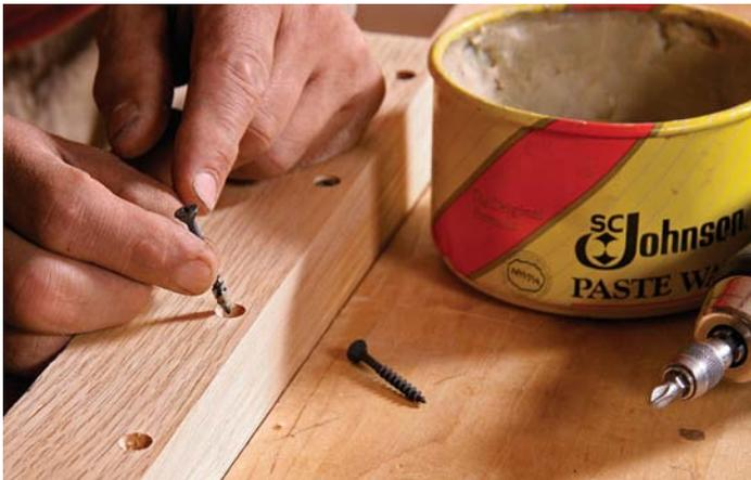
**Wax works.** Rub a little paste wax or paraffin on the threads to coax a screw into place more easily.
