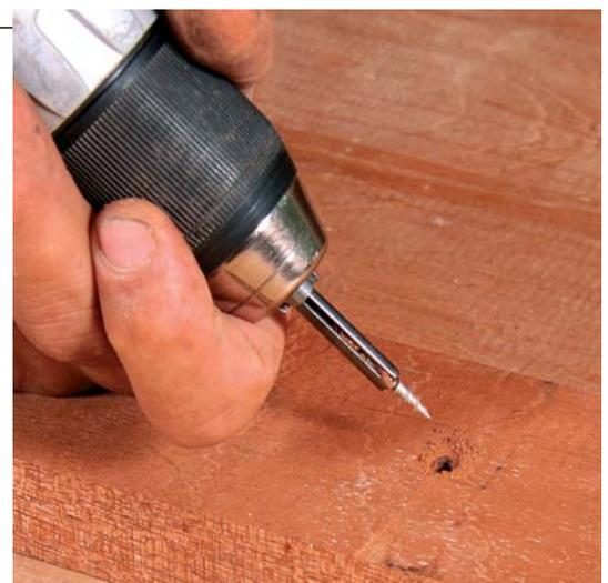
**Simple extraction.** With one of the extractor sleeves in the chuck and his drill in reverse, Rodriguez carefully drills down over the screw (left). The extractor cuts down, tightening around the screw and eventually backing it out of the hole (above).
