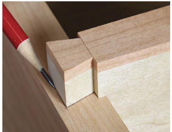
**Trace the tail.** Once the tail is pared, use it for layout. Then saw, chisel, and use a router plane to create the housing.
