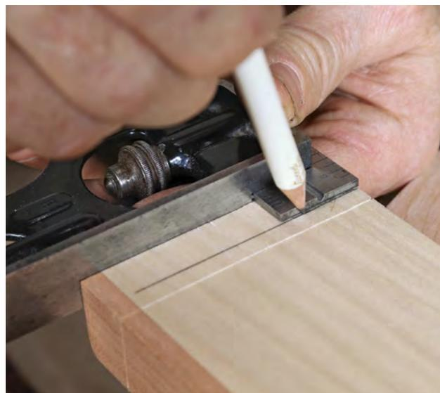
**Determine stub tenon length.** With the divider still in place, pencil the dado depth on the divider (above). This will be the length of the stub tenon. Use a combination square to carry the line across the divider (left).
