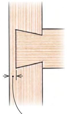
with the inside of the case. The steps used to cut each of these are similar. They all start with cutting dados in the case and trimming the dividers to length. Then, after making the dovetails (and, if necessary, tenons), you'll tap in the dividers and trace the tail onto the front edge of the case side. From there, it's a matter of using a saw, chisels, and a router plane to form the dovetail housing.
