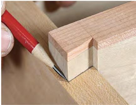
**Trace the dovetail onto the case side.** The stub tenon registers in the dado, ensuring the divider stays put. Trace around the tail with a pencil, then scribe the lap with a marking gauge.
