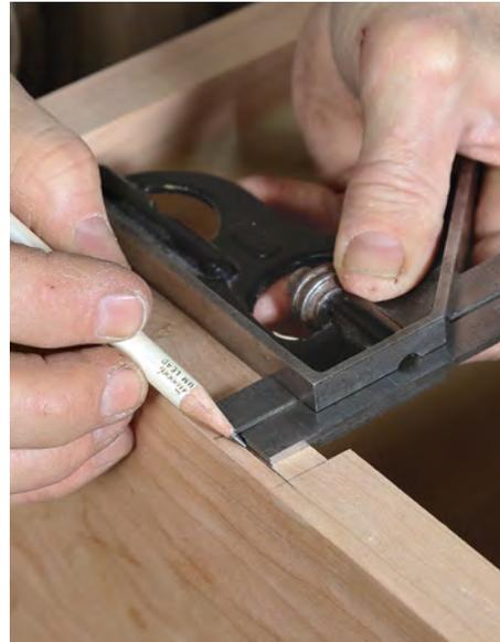
**Lay out the dovetail housing.** Use a combination square to mark the length of the dovetail on each case side.
