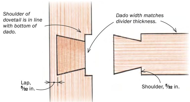
part of the joint much easier to cut. I use a router plane to bring each housing to a consistent depth, helping with repeatability.
