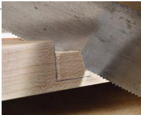
**Saw out the housing and chisel to your lines.** To clean up the bottom of the housing, use a chisel (right) or a router plane.
