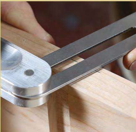
**Transfer the dovetail angle.** Set a bevel gauge to the angle of the tail. Tilt the tablesaw blade to match.
