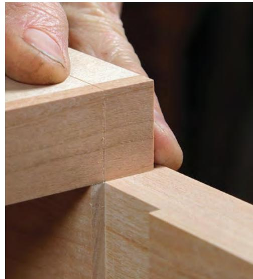
**Mark the dovetail length.** The shoulder of the tail should align with the bottom of the dado. Neptune sneaks up on this dimension with a marking gauge at the back edge of the divider to keep the show edge clean.
