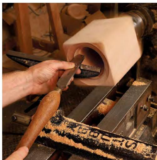
**The sides get scraped smooth.** With the hollowing virtually finished, Gardner switches to a straight scraper to smooth the sides of the cavity.
