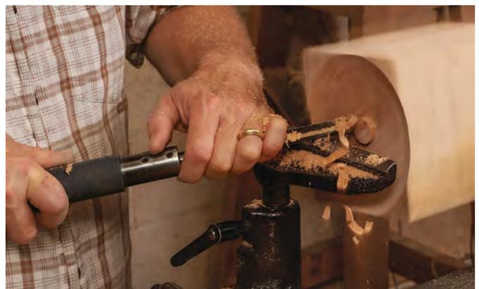
**Dish out the underside.** Using a  $\frac{1}{2}$ -in. bowl gouge, cut a concave recess on the bottom of the blank. Leave wood at the corners, as they will be the feet of the box.
