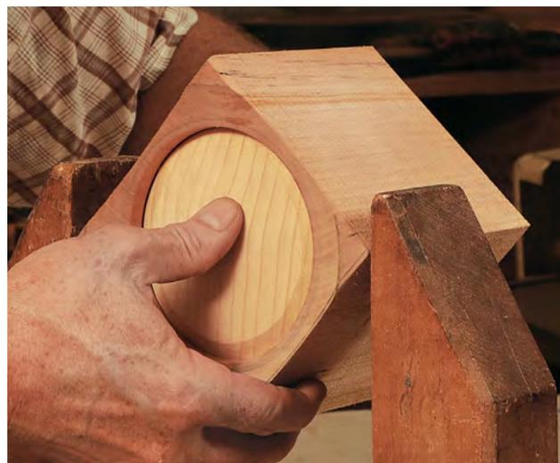
**Pop it in place.** With the box body back in the hand-screw clamp, Gardner tips the bottom into its groove and gently pushes until it pops into place. Then he removes the clamp and sets the box aside to dry for several weeks.
