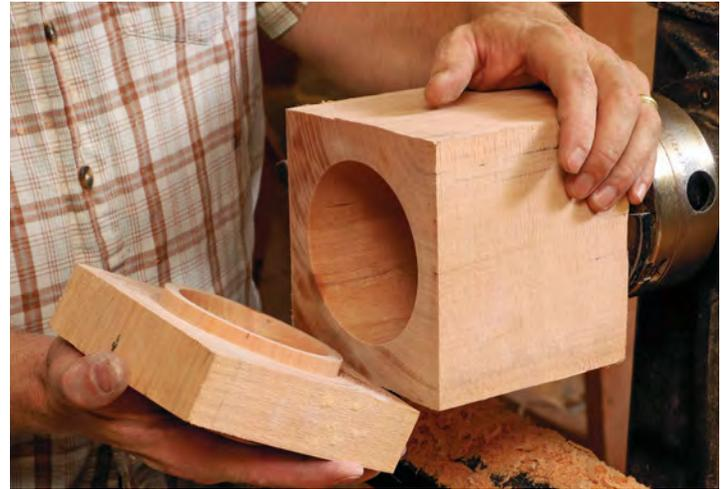
**Fit the lid.** Mount the body on the jam chuck and put the lid in place.
