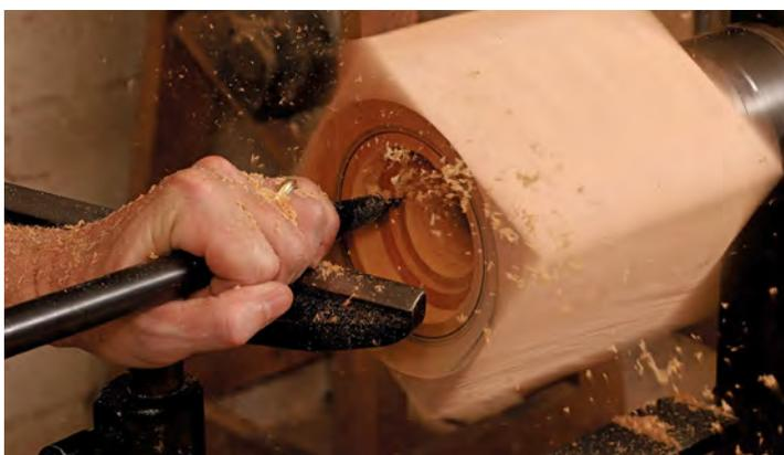
**Open up the inside.** Gardner does most of the excavation with a hollowing tool fitted with a  $\frac{3}{16}$ -in. round-nosed scraper-style cutter. The work goes quickly as he widens the drilled hole. He stops when he has nearly reached final wall thickness.
