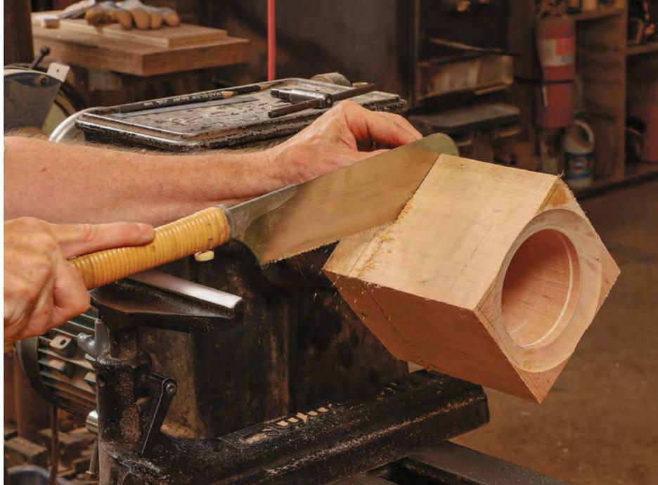
**Saw through from there.** Finish the separation safely with a hand saw and the lathe turned off to avoid having the body of the box fly off the lathe.
