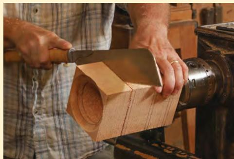
**Parting off the bottom box.** After hollowing the bottom box to the depth of the drilled hole, use a parting tool and then a hand saw to separate it from the rest of the blank.
