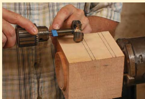
**The second story.** Once the bottom box is parted off, Gardner turns a tenon on the next box up that will register it on the bottom one. Next he'll drill and turn the cavity in the second box.
