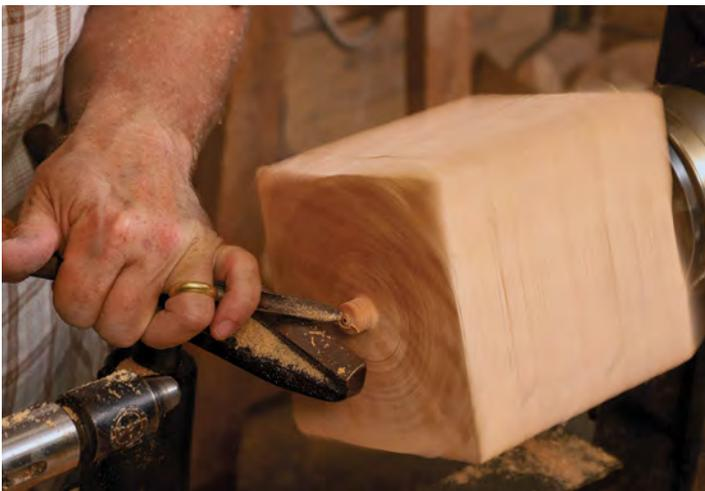
**Tenon removal.** With the lid fitted onto the body, turn away the tenon and give the top a very slightly domed surface. For most of this step, use the tailstock with a live center to support the lid; back it off at the end to remove the small plug of wood at the center.
