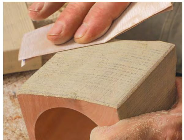
**Sandpaper exposes the undercoat.** When the topcoat is dry, Gardner sands the textured surface, revealing the darker undercoat on the high spots where the topcoat is rubbed away.
