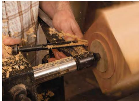
**Start with a spigot.** With the blank between centers, turn a tenon on its top end (left) to fit a four-jaw chuck (below).
