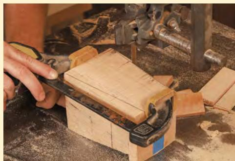
**Tapering the tower.** Gardner bandsaws the whole stack to a taper. After sawing two sides, he tapes an offcut from the lid back in place; that holds the stack in position while he cuts the last two sides.
