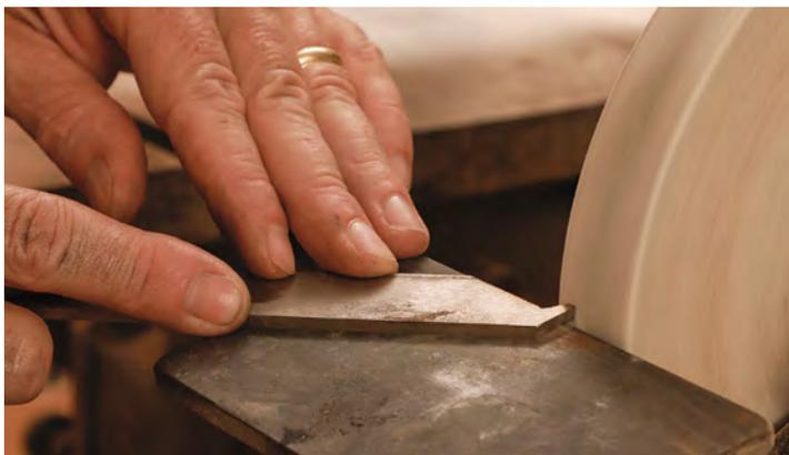
**Custom-made grooving tool.** To cut the groove for the box bottom, Gardner made a special tool from an old planer knife. He roughed out its shape with an angle grinder and refined it on the grinding wheel. To see how he made it, go to [FineWoodworking.com/304](http://FineWoodworking.com/304).
