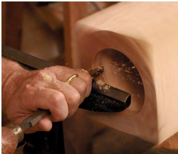
**Clean shoulders.** After mounting the body in the jam chuck, flatten the top face and smooth the top section of the interior wall.
