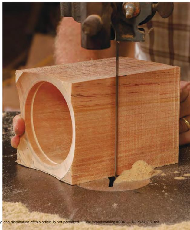
**Bandsawn texture.** With the box held at an oblique angle to the bandsaw blade, Gardner draws the box toward the teeth, creating a scratchy texture. He then stands the box upright and repeats the process to produce a crosshatched effect.
