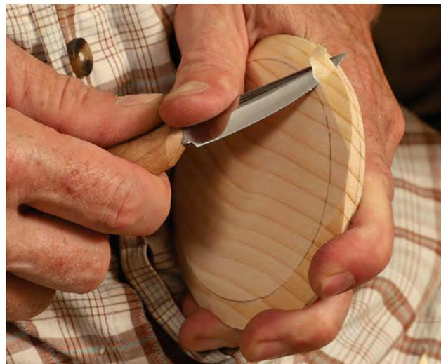
**Saw and slice.** Gardner cuts carefully to his perimeter pencil line at the bandsaw, then draws two more layout lines: one on the bottom face  $\frac{1}{2}$  in. from the outside edge, the other around the edge,  $\frac{3}{8}$  in. down from the top face. Using a sloyd knife, he connects the layout lines to create an underbevel.
