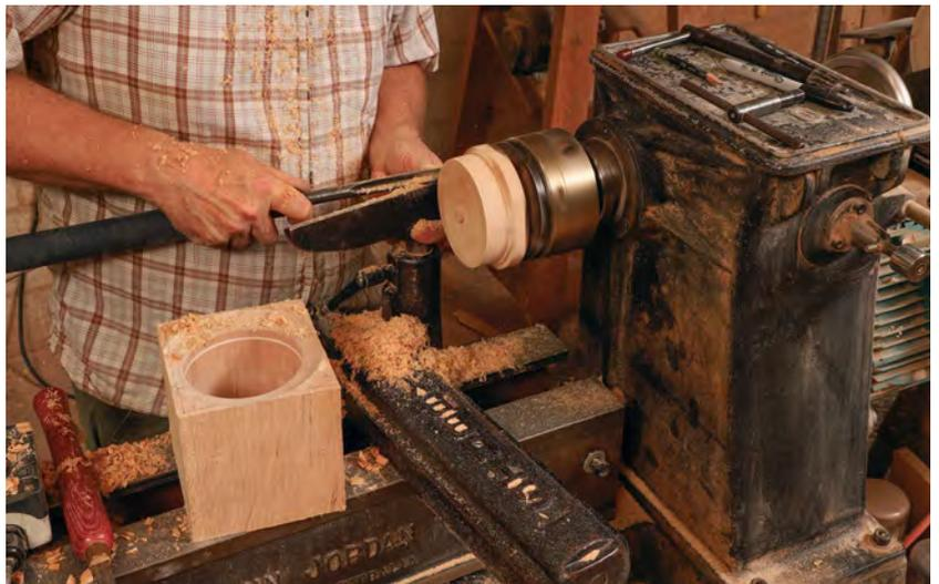
**Remounting the body.** With the lid separated and removed from the lathe, turn a jam chuck to fit the bottom opening of the box body.
