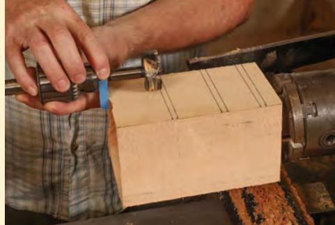
**Hollow one layer at a time.** After turning a tenon on the top of the box blank, mount it in a four-jaw chuck and drill deep enough for the bottom box.
