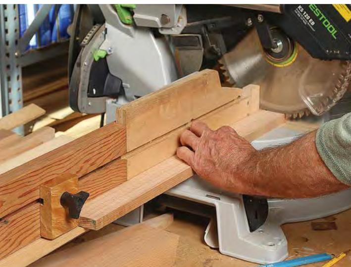
**Stationary fence with extension.** An auxiliary fence with a replaceable zero-clearance throat piece and a groove for an adjustable stop are the foundation for straight, square, repeatable cuts, without tearout. The removable extension fence locks onto either end of the stationary fence via dowels. It also has a ledge on the bottom to support the workpiece at the same height as the saw's table.
