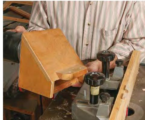
**Dust be gone.** The shopmade fence has—you guessed it—a replaceable, zero-clearance insert. It makes for safer and cleaner cuts and also helps control dust and shavings, which pass into a shopmade dust hood. The dust hose plugs into a port in the back of the hood.
