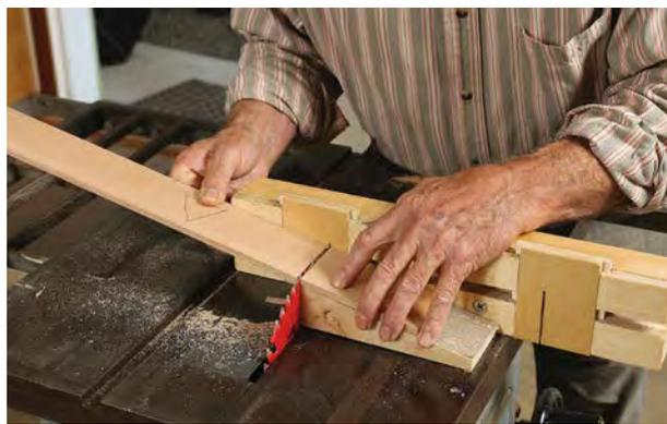
**Versatile auxiliary fence.** The shopmade add-on to the saw's miter gauge prevents tearout by backing up the cut with a replaceable insert. It also has an easily adjustable stop. A simple ramp held against the fence aids in crosscutting angles.
