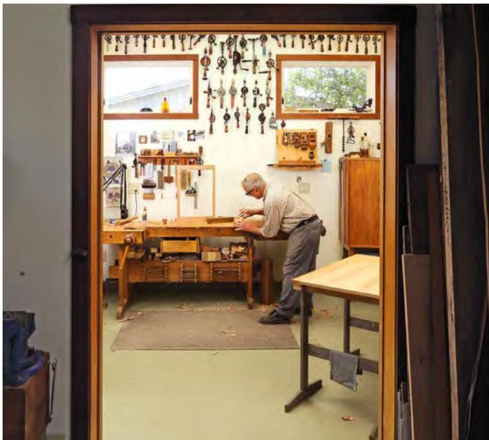
**Big enough.** Just over 150 sq. ft. with high ceilings and lots of windows, the bench room has enough space for a large bench, storage cabinets, lots of light, and open floor space for gluing up larger pieces and working on pieces in progress. The floors are gentle on the body, poured concrete with multiple layers of plywood on top and vinyl flooring tops it off.
