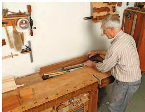
**Bench upgrades.** Trough covers, level with the bench's surface, provide easy-access storage. Long ago, James Krenov installed holders for rasps and files on the front of the bench (below). It's easy to see the one you want and grab it.
