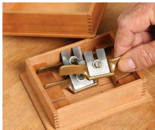
**Custom tool boxes.** Welter makes custom boxes for hand tools that are special or seldom used. He tailors the size of the box and the cradles inside to the specific tool, and stores the boxes on a shelf.
