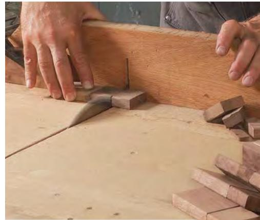
**To length.** At the table saw, crosscut the glued-up pairs of full tiles to make the one-and-a-half-length tiles.
