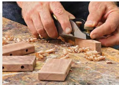
**Angled edges.** Make the initial bevel cut at the bandsaw with the table tilted, then smooth the sawn surface with a block plane.
