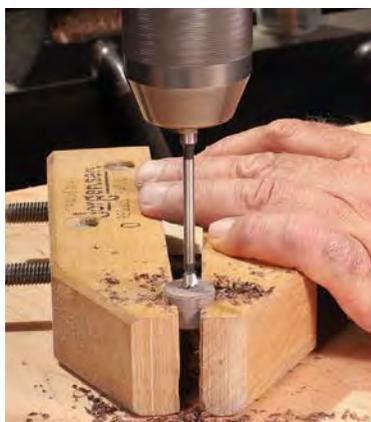
**Custom clamping.** To hold a bead securely while drilling through it, you can customize a hand-screw clamp: use a Forstner bit to cut a shallow hole in the jaws to fit the bead.
