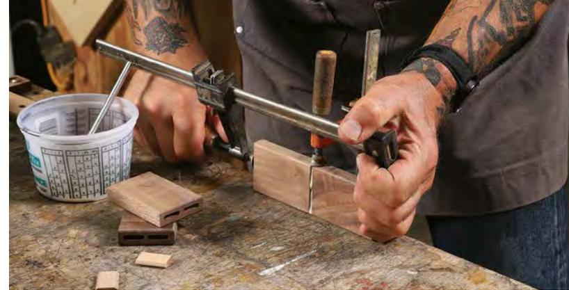
**Glue two full tiles end to end.** Before mortising and gluing up the paired tiles, round over their edges at the router table. Clean the squeeze-out at the glue joint with a damp rag.
