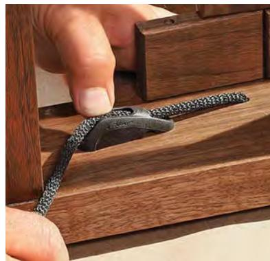
**Cleat tightening.** With the rope pulled through to the inside, cinch it tight in the rope cleat. Then cut off the excess rope and torch the end.
