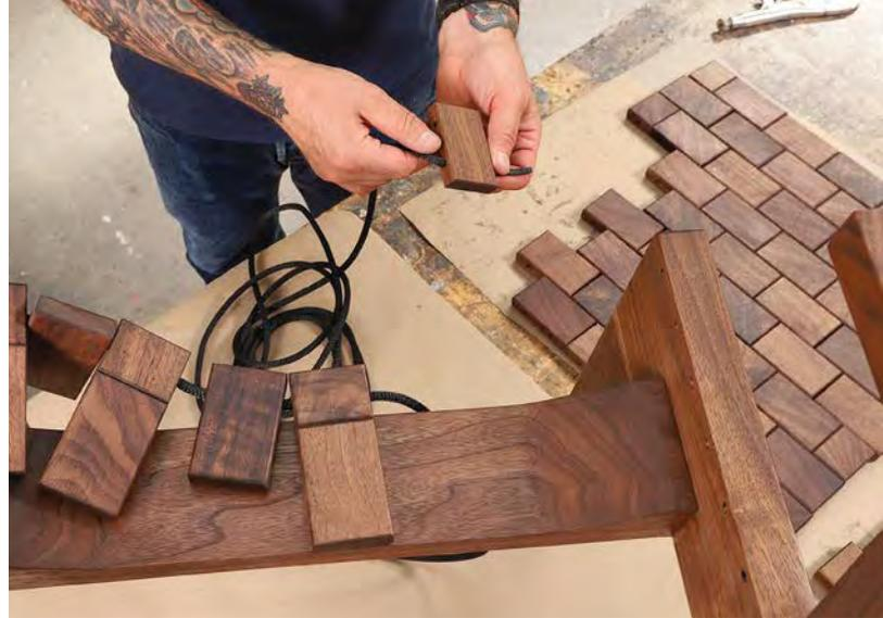
**The running bond begins.** After tying a square knot at one end and passing the rope through the first hole at the front of the seat, thread on nine tiles to make the first row, alternating full-length and one-and-a-half-length tiles.
