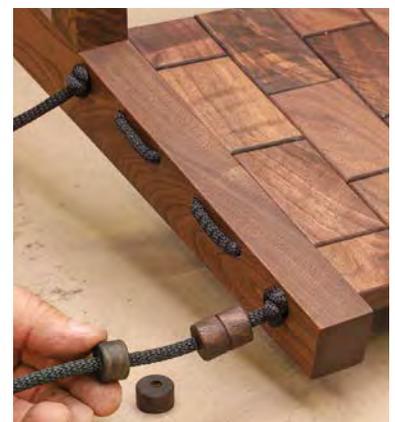
**Thread the beads.** Lace on a few beads to decorate the top knot of the chair's back. Then tie off the rope, cut it, and torch it.
