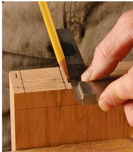
**Mark the widths of the tails on the end.** Set the pencil point into the depressions from the points of the dividers, slide a square up to the pencil point, and draw lines across.
