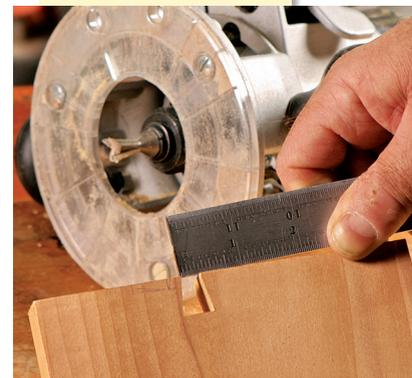
**Sizing pins for router-cut dovetails.** If you plan to cut dovetails with a router, the minimum pin width will be dictated by the diameter at the base of the bit.
