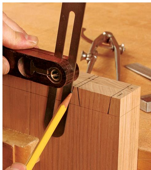
**Mark the tails on the face.** Use the bevel gauge to draw in the tails on the face of the board.
