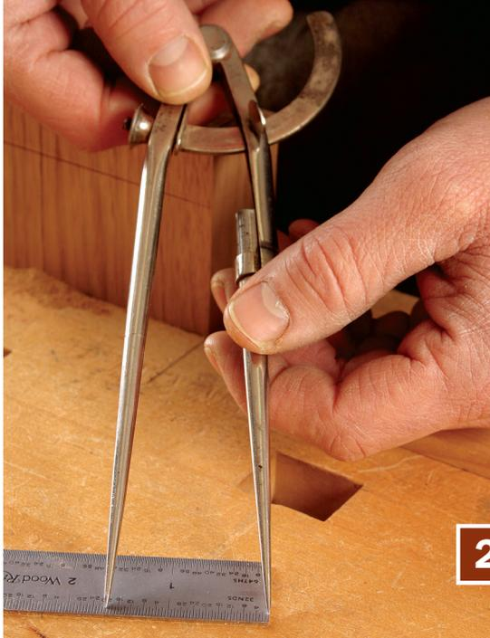
**2** **Measure from the half-pin mark on one end to the pin-width mark on the other.** Divide that distance by the number of tails; adjust the dividers to this dimension.
