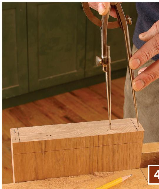
**4** **Mark the right edges of the tails.** Repeat the process beginning from the left half-pin line.
